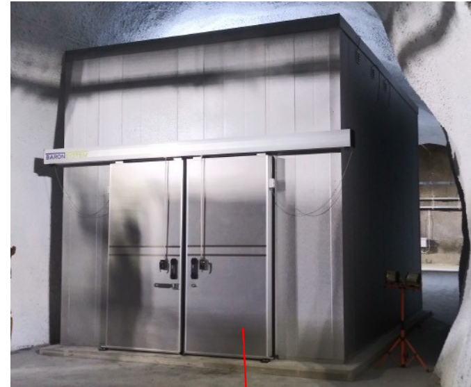
Shielding base for muon detector
