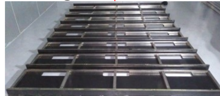
Shielding base for muon detector
